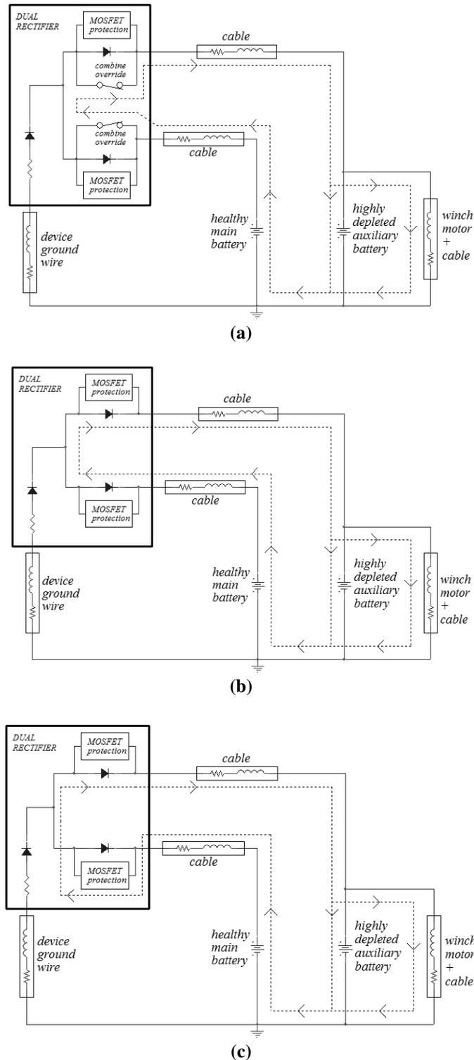
**Figure 2: Reverse current turn-off transient behavior in combine mode with system loop inductance. (a) Main battery supplying current to depleted auxiliary battery and winch motor (main diode functionality overridden). (b) Reverse current during MOSFET array turn-off. (c) Reverse current flowing through the main MOSFET array protection circuitry and auxiliary MOSFET array due to system inductance.**
