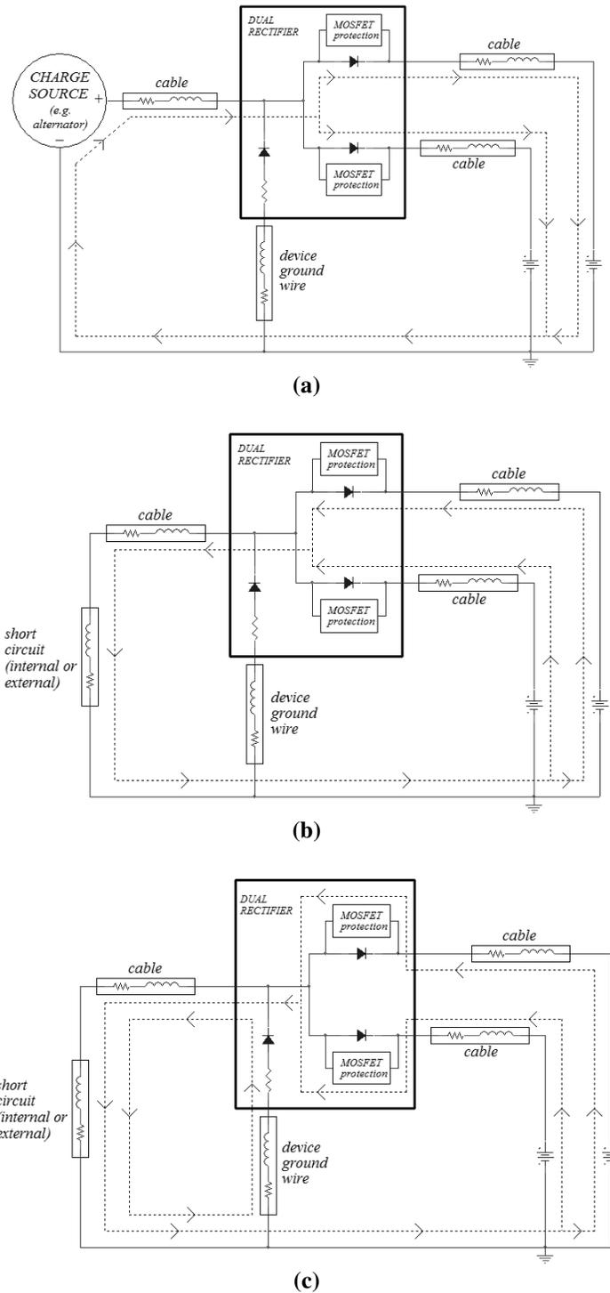
**Figure 1: Reverse current turn-off transient behavior in normal diode mode with system loop inductances.**
