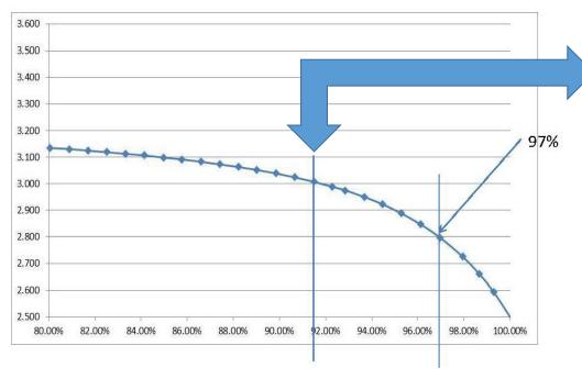
LiFePO4 Power-Type Cell Discharge Curve (Per Cell)
