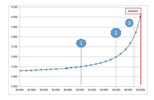
LiFePO4 Power-Type Cell CHARGE Curve (Per Cell) Point 2 to Point 3:
