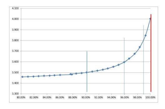
LiFePO4 Power-Type Cell CHARGE Curve (Per Cell)
