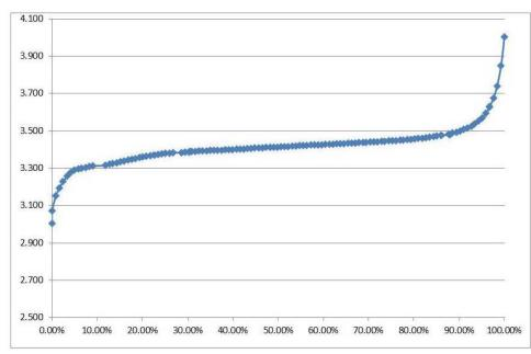
LiFePO4 Power-Type Cell CHARGE Curve (Per Cell)
