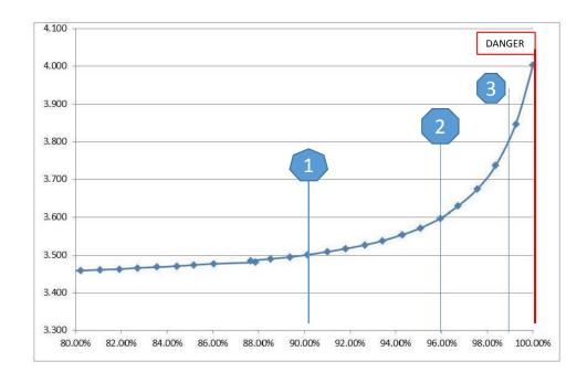
LiFePO4 Power-Type Cell CHARGE Curve (Per Cell)
