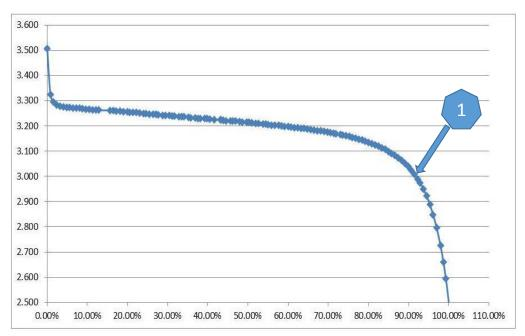
LiFePO4 Power-Type Cell Discharge Curve (Per Cell)
