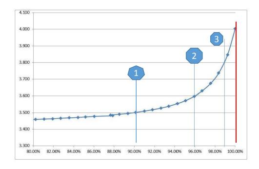
LiFePO4 Power-Type Cell CHARGE Curve (Per Cell)
