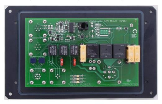
The replaceable fuses are shown in the internal view of the Model 290 Engine Interface. Access to the fuses is possible by removing the 4 screws that attach the cover to the main panel.
