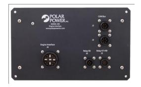
Through software, the 8 on board relays and 3 switch inputs can be assigned various functions encompassing: engine speed control, fuel valves, cooling and ventilation fans, engine block heaters, fuel heaters, safety shut down devices, and the normal functions required by a diesel or LPG fueled engine.
