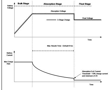
**NOTE**: When the charge cycle is interrupted, the charger will restart charging at the beginning of the multistage algorithm. Charge current during equalize state (optional state not shown here) is normally limited to 10A for 60 minutes.
