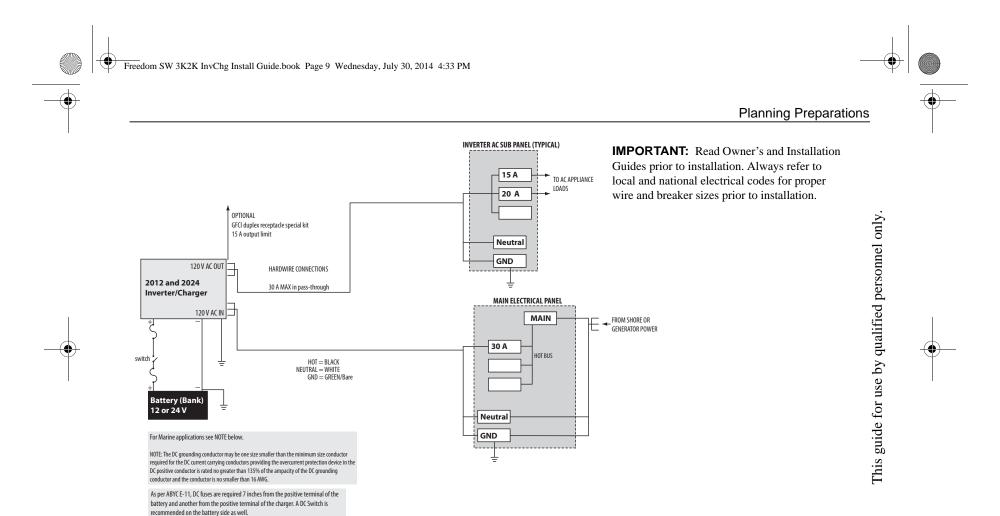
Figure 4 Wiring and Breakers Block Diagram for Freedom SW 2012 / 2024
