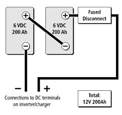
Figure 24 Batteries Connected in Series
