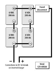
Figure 25 Batteries in Series-Parallel Connections
