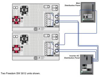
Figure 21 Neutral Wiring for Stacking
