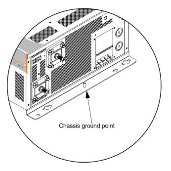
Figure 10 DC Wiring and DC Grounding
