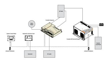
Figure 2 Typical Xanbus System Diagram
