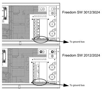
Figure 7 AC Wiring Compartment
