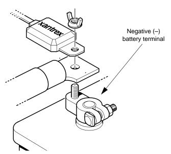
Figure 12 BTS Mounted on the Negative Battery Terminal
