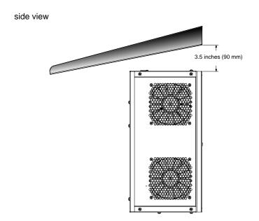
Figure 27 Drip Shield Placement (Inverter Front Panel Facing Up)
