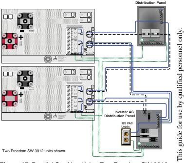
Figure 17 Parallel Stacking Using Two Freedom SW 3012s
