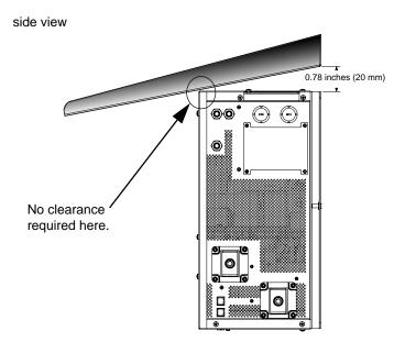
Figure 28 Drip Shield Placement (Inverter Front Panel Facing Down)
