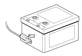
Figure 14 BTS Mounted on the Battery Case
