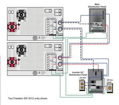
Figure 18 Series Stacking Using Two Freedom SW 3012s
