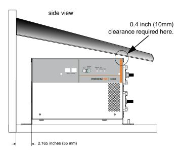
Figure 26 Drip Shield Placement (Desktop Mount)
