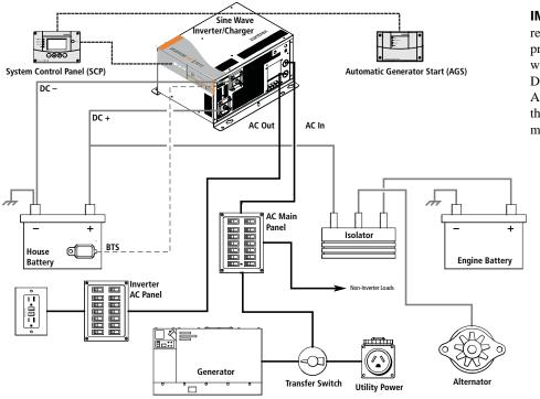
**IMPORTANT:** Figure 3 does not show all required grounding or overcurrent protection. See the following two pages as well as page 17 for information on required DC grounding or overcurrent protection. Always hire a qualified personnel to ensure that all electrical safety requirements are met before, during, and after installation.
