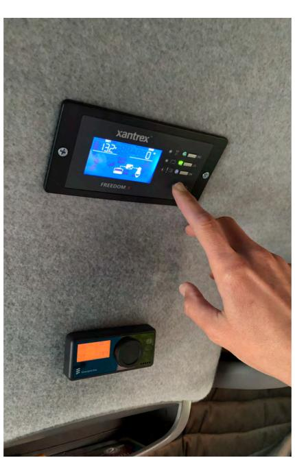
Remote panel for Xantrex Freedom XC 2000 installed overhead, in cab headliner. Inverters are best kept "OFF" when not in use. Thus, a highly visible location (such as this) is ideal.
